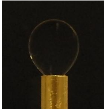
Figure B.3: The photograph of the PDMS droplet surrounded by water, used in determining the interfacial tension between the two.
