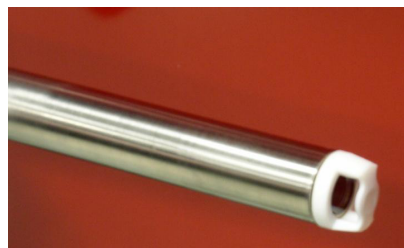
Figure 3.26: The reflector cap of the PVM ® for reducing light reflectance from droplets (Image from Mettler Toledo ® brochure).
